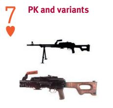
Type: General-purpose machine gun Calibre: 7.62×54R mm Distinguishing features: Oval hole in stock; triangle profile front sight
