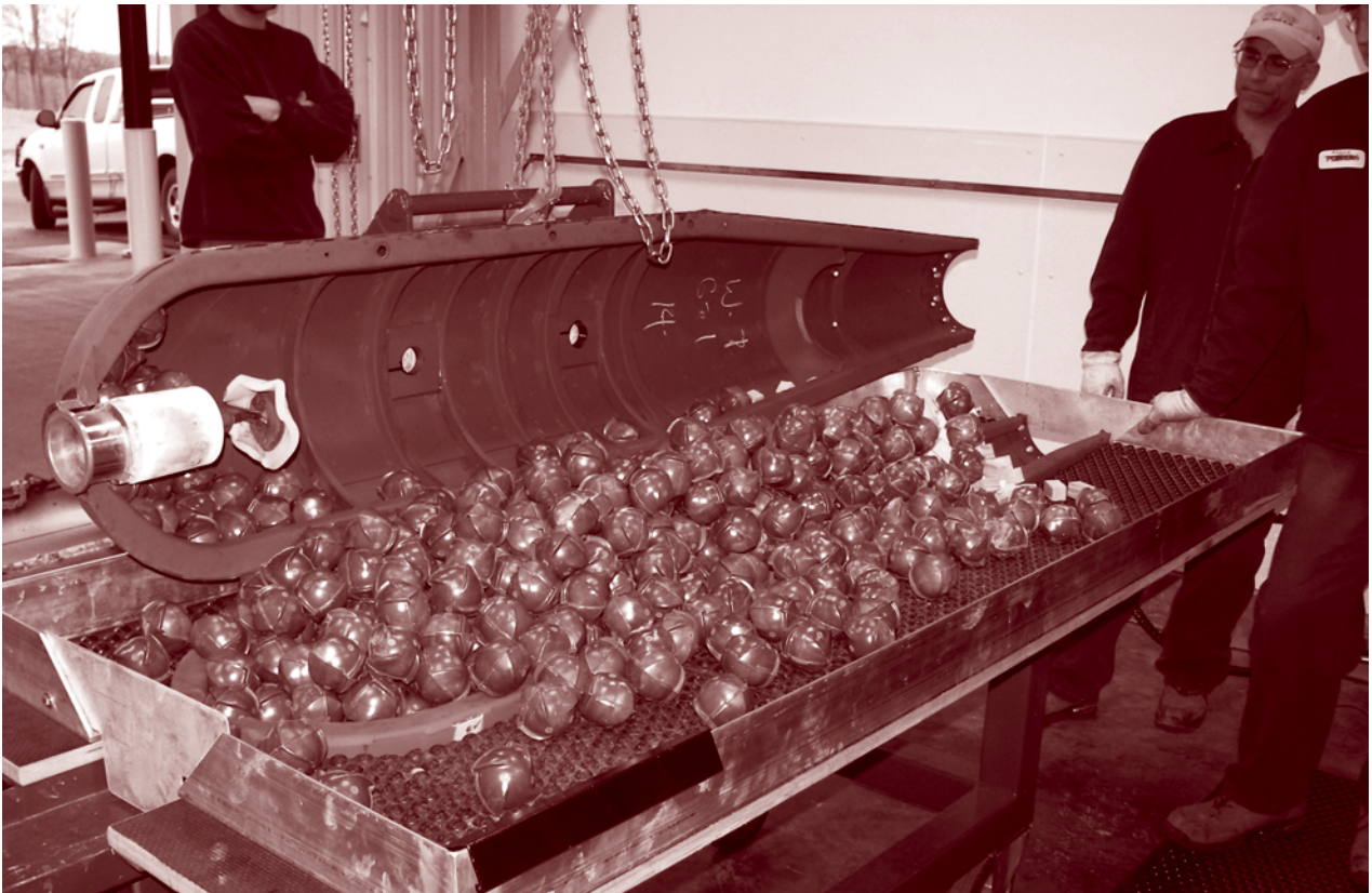
CBU bomblets undergo an automated demilitarization process at Joplin, Missouri, USA, 2012. © General Dynamics Ordnance and Tactical Systems (GD-OTS)
