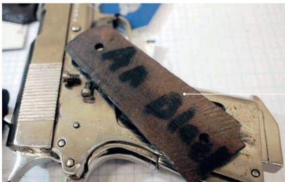
Handsaw marks evident on the underside of the wooden grips
