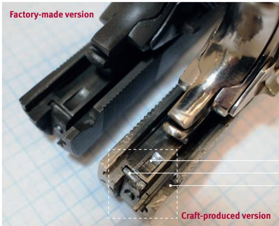
Hand-tooled characteristics such as coarse and uneven toolmark stripe, and poor overall finish
