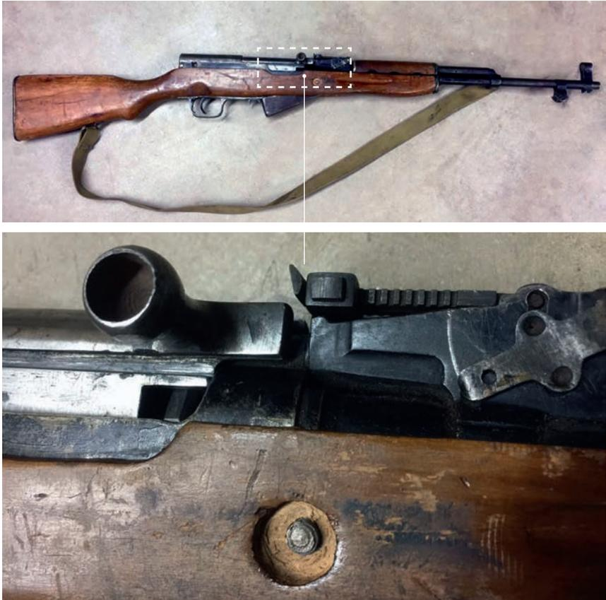
Note: The close-up image shows the poor fit, crude finish, and obvious tool marks.
