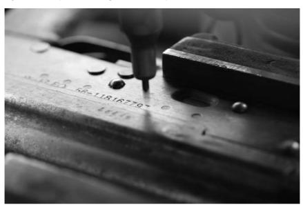
Figure 1 A dot-peen marking machine in operation
