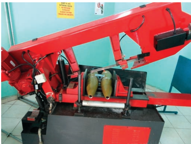
High-explosive projectiles being processed using an industrial bandsaw (left), and the resulting opened shells being transported for the removal of energetics (right). © NAMSA
