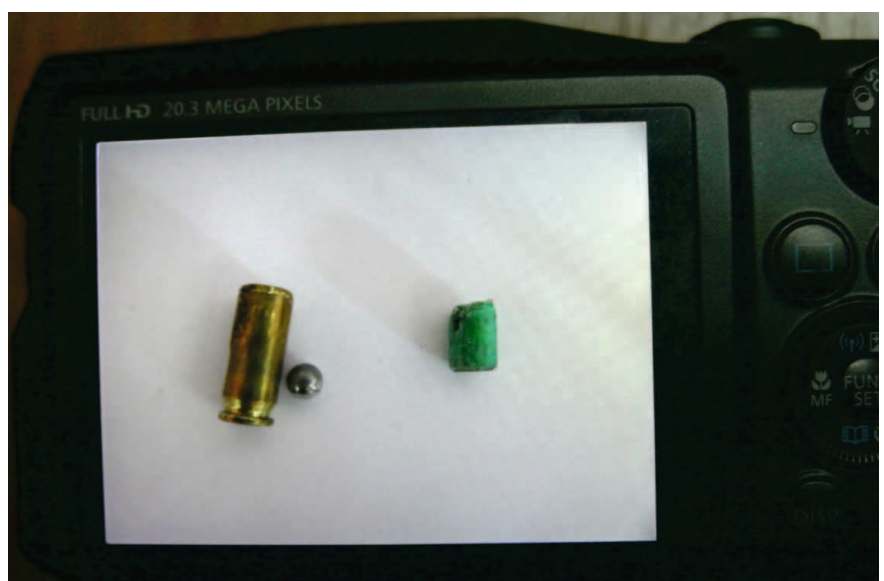
Post-test firing of a converted Ekol Tuna alarm pistol: cartridge case, steel ball, plastic wadding. Nouakchott Police Forensic Science Service, December 2017. Source: Mauritania National Police Forensic Science Service
