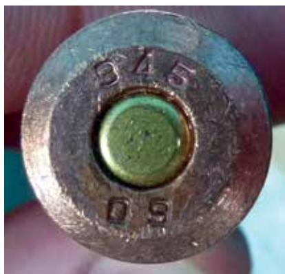
Photo 4: A Factory 945 7.62 × 54R mm cartridge produced in 2009 and found in Sudanese packaging. The SPLA captured the rounds from Athor's SSDM/A in March 2011. Jonglei, South Sudan, April 2011. © Jonah Leff
