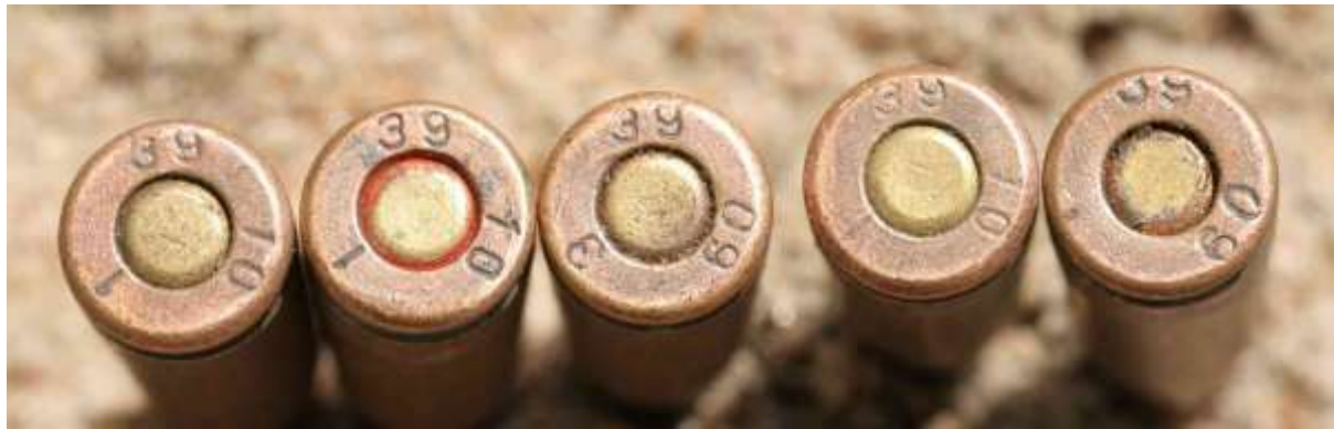
Sudanese-manufactured 7.62 x 39 mm ammunition found loose (unboxed). The ammunition headstamp features three entries: calibre ('39'), date ('10' or '09'), and what appears to be a lot or batch designator ('1' or '3'). Date marks suggest the ammunition was manufactured in 2009 and 2010. For further information, see the HSBA publication 'A Guide to Sudanese Ammunition (1954-present).' The Small Arms Survey has observed similar varieties of ammunition throughout Sudan and South Sudan.
