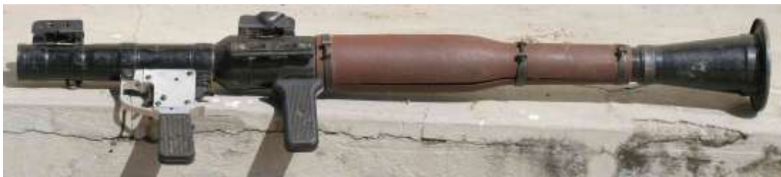
Sudanese manufactured RPG-7-type rocket launcher reportedly seized from Duit's forces. The weapon is of quite crude construction and differs from most known models in use in the region (Chinese, Russian, Iranian). The trigger assembly is similar to that of Bulgarian models (there is not a chamfered cutaway to the rear of the aluminium trigger assembly). The plastic heat shield resembles Iranian variants, but differs in colour. Identical launchers have been recovered from George Athor's forces in 2011, from Darfurian rebels in 2010 and from Al Shabaab in Somalia in 2011.
