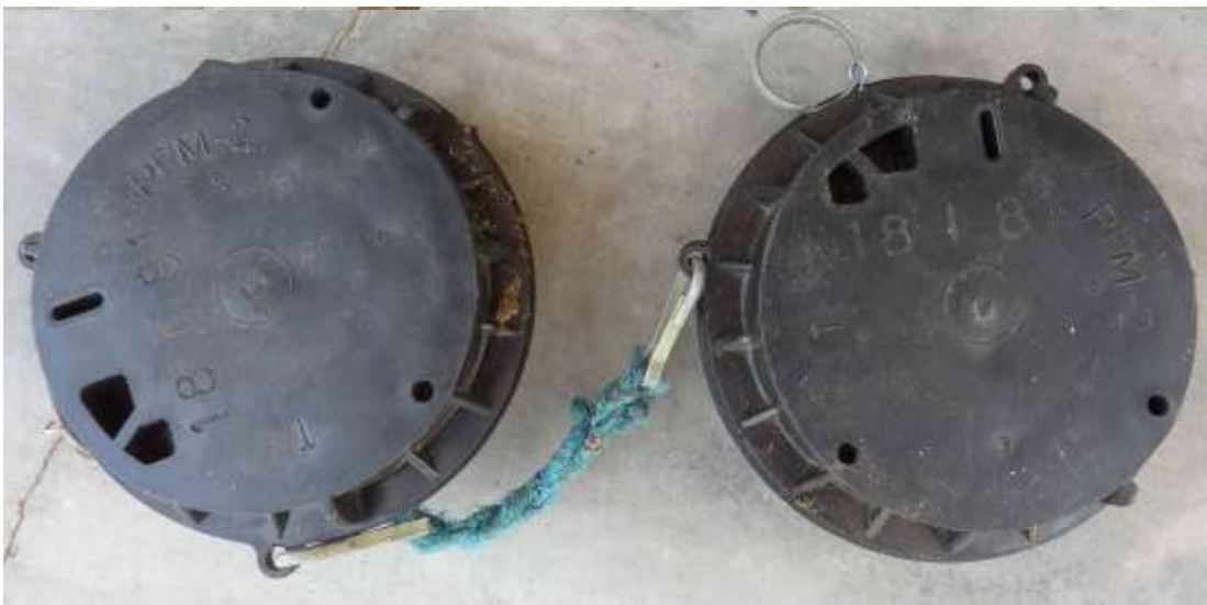
PPM-2 anti-personnel mines reportedly seized from Athor's forces. Upper image: top surface of the mines. Lower image: underside of the mines, illustrating the model designations ('PPM-2') and lot codes ('18181') in each example. The design, construction, and marking of the mines are consistent with former East German (GDR) manufacture.
