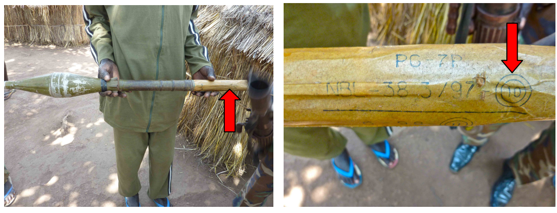
PG-7P propellant charge manufactured in Bulgaria in 1997 (left and right photos). The encircled '10' denotes Bulgarian production.
