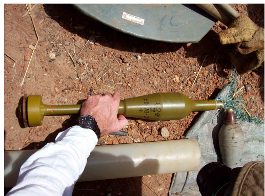
Chinese manufactured Type 65 82 mm recoilless rifle round in brand new condition, bearing lot number 50-78-74. This type of ammunition is typically employed against armoured vehicles. This is the first time the Small Arms Survey has observed this type of ammunition in Sudan.
