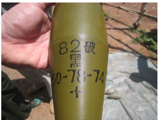
Chinese manufactured Type 65 82 mm recoilless rifle round in brand new condition, bearing lot number 50-78-74. This type of ammunition is typically employed against armoured vehicles. This is the first time the Small Arms Survey has observed this type of ammunition in Sudan.
