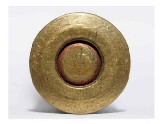
This ammunition closely resembles the previous entry, but is 7.62 x 54R mm in calibre. The cartridge also features a brass case, steel-jacketed lead core bullet, and red primer annulus. The provenance of the ammunition is unknown.
