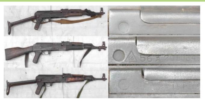
These weapons are clearly old and well used. Factory marks and serial numbers (right-hand images) are heavily weathered through use and abrasion rather than intentional removal.
