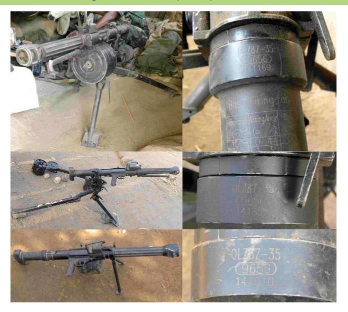
The Small Arms Survey observed three Chinese-type QLZ-87 35 mm automatic grenade launchers in South Kordofan and Blue Nile. According to marking codes visible on various parts of the launchers, they were all manufactured by the same producer (identified by the '9656' code). The relatively close sequence of serial numbers suggests that these three launchers were most likely part of a single consignment.
