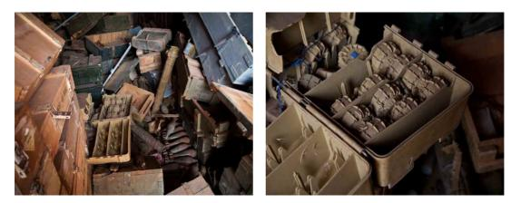
A box of AP mines resembling the Italian manufactured TS-50 and VS-50 varieties. The VS-50 is also manufactured under license as the SPM-1 in Singapore. Other variants include the Egyptian-produced T-79 and the Iranian YM-1/1B. It is unclear whether the SPLA or JEM confiscated these mines.
